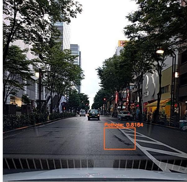
**Figure 16.** Object detection system detects potholes.
