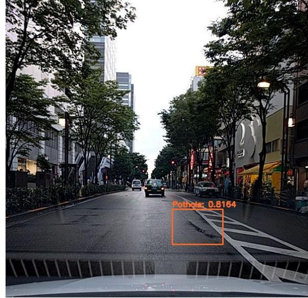
**Figure 16.** Object detection system detects potholes.
