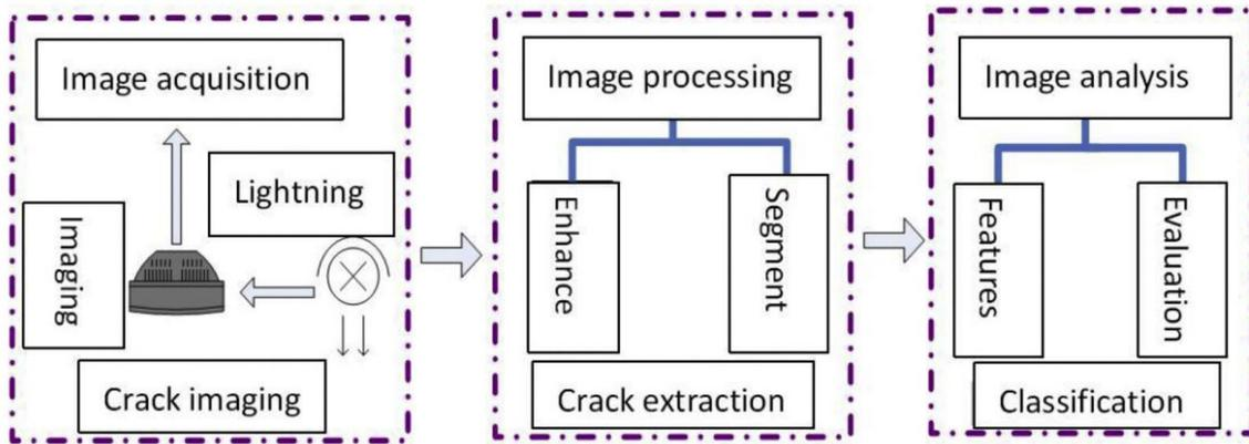
**Figure 17:** Diagram of Crack Detection System
