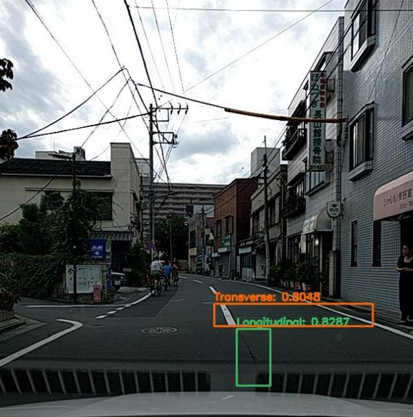
**Figure 15.** Object detection performs system transverse and longitudinal crack detection
